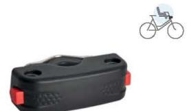
Fits frames from Ø22 to 40 mm. Requires only an available length of 35 mm to be installed. Inside the holder, a rubber pad protects the bicycle and allows the mounting system to adapt to frames of all different sizes. Mounting kit includes two mounting options: one for small head tubes (10 mm / Ø28-40 mm) and another for standard head tubes (35 mm / Ø22-40 mm). Mounting kit required for assembling included. Meets all the safety standards EN 14344. Sold as a spare part.
