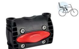
Fits frames from Ø28 to 40 mm. Requires only an available length of 80 mm to be installed. Inside the holder, a rubber pad protects the bicycle and allows the mounting system to adapt to frames of all different sizes. The rear metallic part of the holder has an opening to allow the brake cables to fit in without being pinched. Meets all the safety standards EN 14344. Sold as a spare part.
